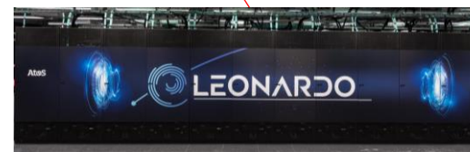
#4, ~240 PF HPL , 2023, 7,5 MW , Leonardo ( EuroHPC ), CINECA, Italy, Atos XH2000 , ~14K Nvidia A100
