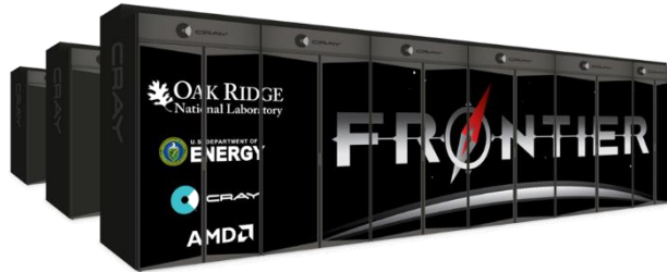
# 1, Frontier, 1.2 EF HPL , 2022, 22MW , Oak Ridge National Laboratory (ORNL) HPE Cray , ~38K AMD MI250X
