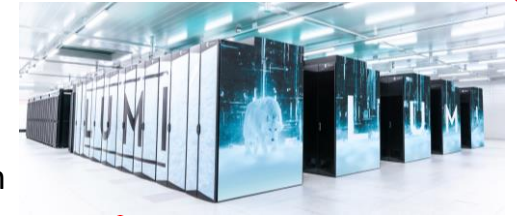
# 3, LUMI-G ( EuroHPC ), ~310 PF HPL , 2023, 6 MW , CSC, Finland, HPE Cray , ~10K AMD MI250X
