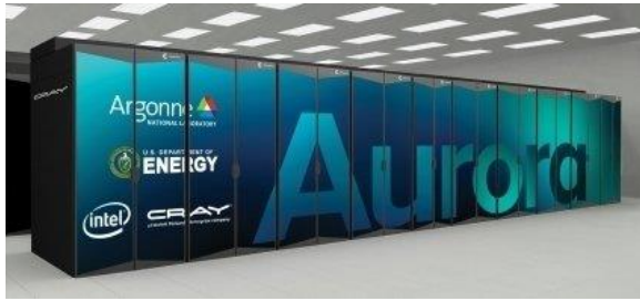
Aurora, >2 EF peak , Q3/2023, Argonne National Laboratory, HPE Cray , ~65K Intel GPU Max , 21K Intel Max CPU
