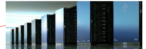
#2, Fugaku, ~440 PF HPL , 2020, 30 MW , RIKEN Center for Computational Science, Japan. Fujitsu A64FX 7,630,848 cores
